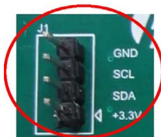
Figure7. I2C Pins Location on PI3EQX1204-AZHE miniSAS EVB
